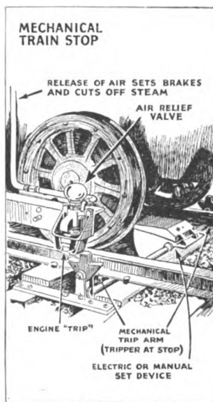
Mechanical Automatic Train Stop in Which a Tripping Device on the Track Is Set Manually or Electrically. The Trip Hits the Air Release Valve on the Side of the Engine and Causes the Brakes to Set
