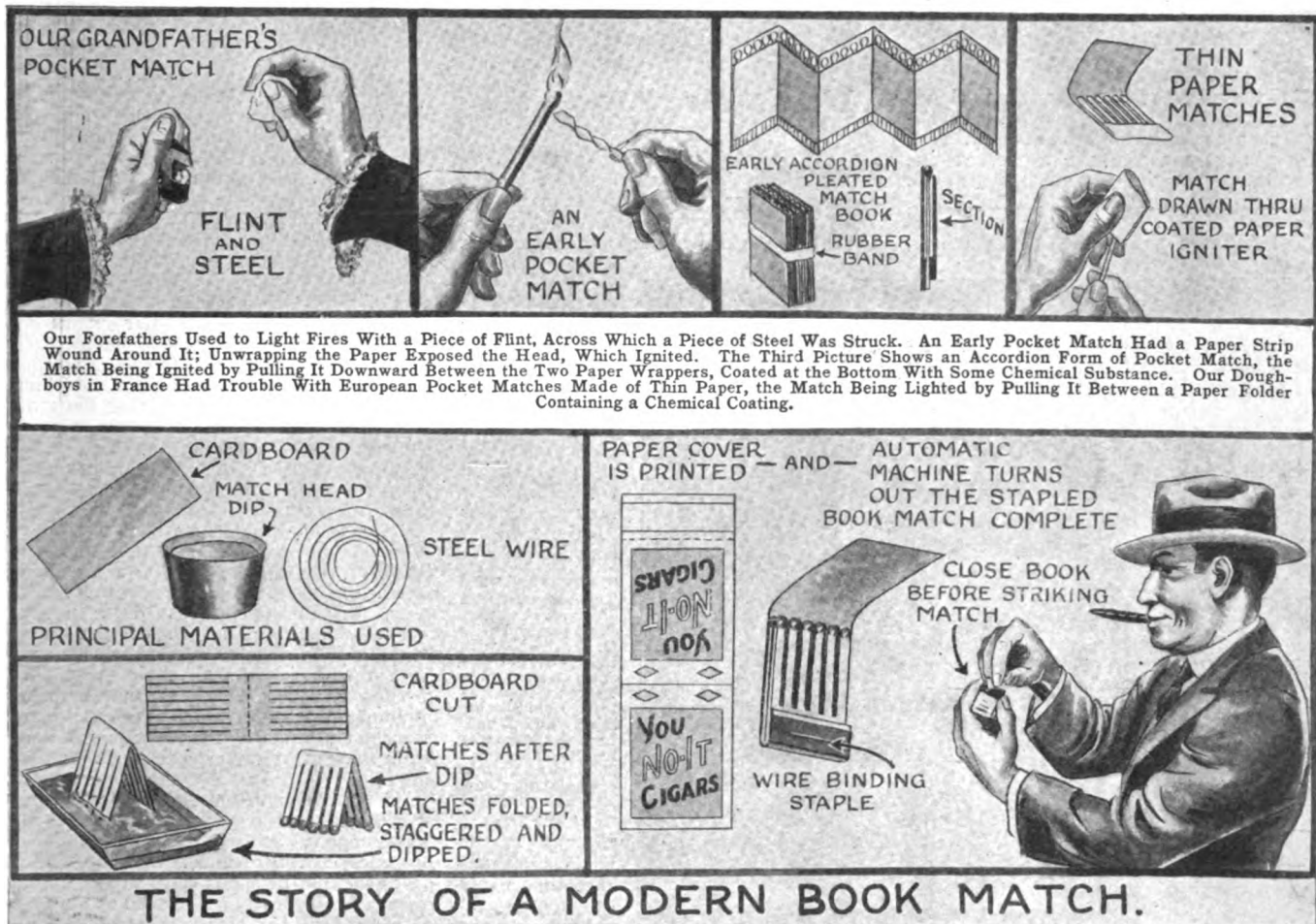
The Book-Match, Which Thousands of Smokers Are Using Everywhere Today, Has an Interesting History. The Early Pocket Matches Were Quite Unsatisfactory, but They Have Improved Marvelously. The Successive Stages in the Making of a Book Match, From the Dipping of the Cardboard Strips to the Printing of the Covers, is Shown in the Series of Drawings at the Bottom, While the Upper Row of Pictures Shows the Forerunners of the Modern Book Match.
